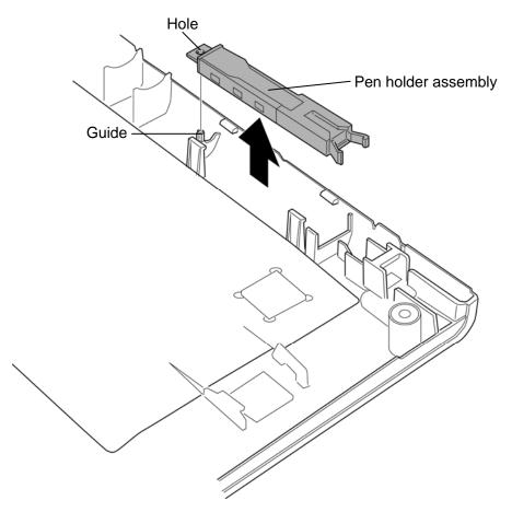
Figure 4-42 Removing the pen holder assembly
